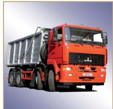
MAZ 8x4 dump truck with 30t payload
